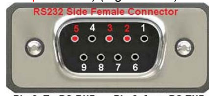
Pin 2: To PC RXD Pin 3: from PC TXD Pin 5: GND
