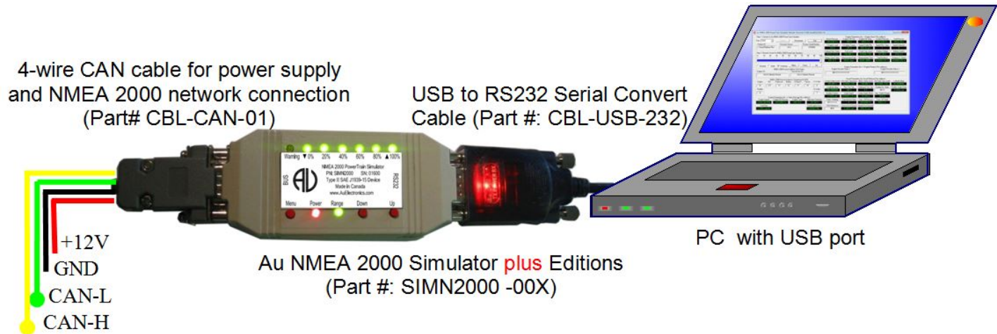
Figure 1-5 Connection of Au NMEA 2000 Simulator plus editions to PC with USB port
