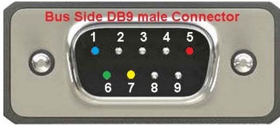
Pin 1: GND Pin 6: CAN-L Pin 5: +12V DC Pin 7: CAN-H
