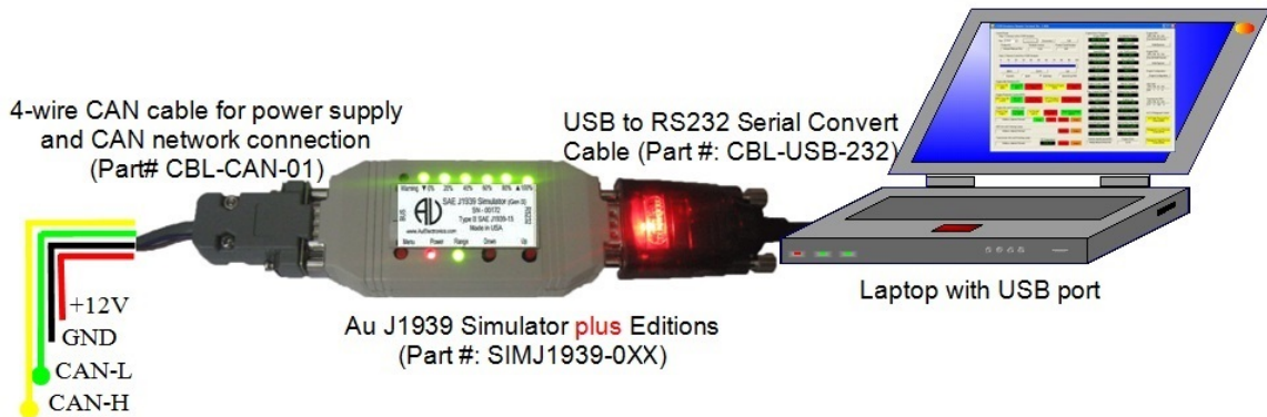
Figure 1-6 Connection of Au J1939 Simulator (Gen II) plus editions to PC with USB port
