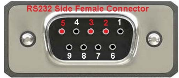
Pin 2: To PC RXD Pin 3: from PC TXD Pin 5: GND
