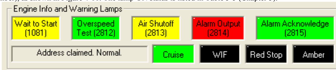
Figure 4-11 Display Engine info and warning lamps
