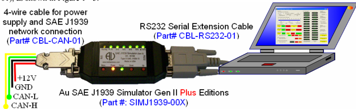
Figure 1-5 Connection of Au J1939 Simulator (Gen II) plus editions to PC with RS232 port
