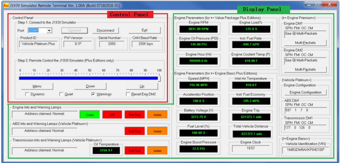
Figure 4-1 Au J1939 Simulator Remote Terminal GUI – Gen II 1.00A Vehicle Platinum Plus Edition
