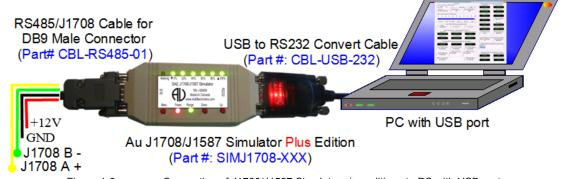
Figure 1-6 Connection of J1708/J1587 Simulator plus editions to PC with USB port
