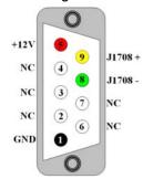
Figure 1-2 BUS Side DB9 male connector
