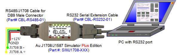
Figure 1-5 Connection of J1708/J1587 Simulator plus editions to PC with RS232 port
