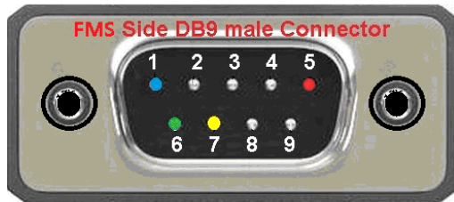
Pin 1: GND Pin 5: +12V DC Pin 6: CAN-L Pin 7: CAN-H
