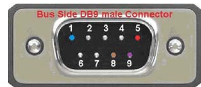
Pin 1: GND Pin 8: J1708- Pin 5: +12V DC Pin 9: J1708+
